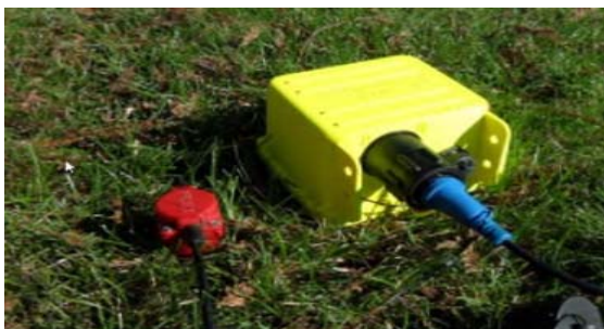
Wireless seismograph for ambient noise tomography
